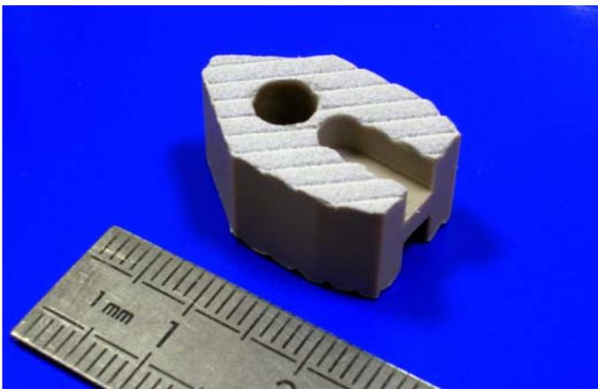
Figure 2: HA coated pure PEEK demonstrator (150  $\mu\text{m}$ ).
