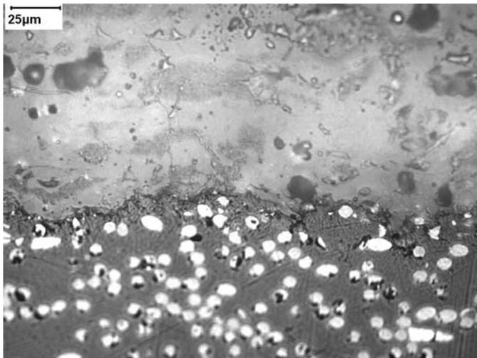
Figure 6: Optical view of the interface between the HA coating and the CF/PEEK substrate.
