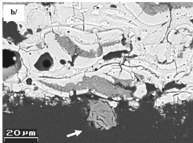
Figure 7a and 7b: BSE views of cross section of HA coating on PEEK (b: alumina particle present at the interface).
