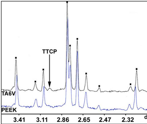
Figure 4: XRD spectrum of hydroxyapatite coating on PEEK and on Ti-6Al-4V (TA6V).
