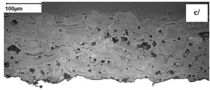
Figure 5a, 5b and 5c: Optical view of cross-sections of a/ HA coating on PEEK; b/ HA coating on CF/PEEK; c/ HA coating on Ti-6Al-4V.
