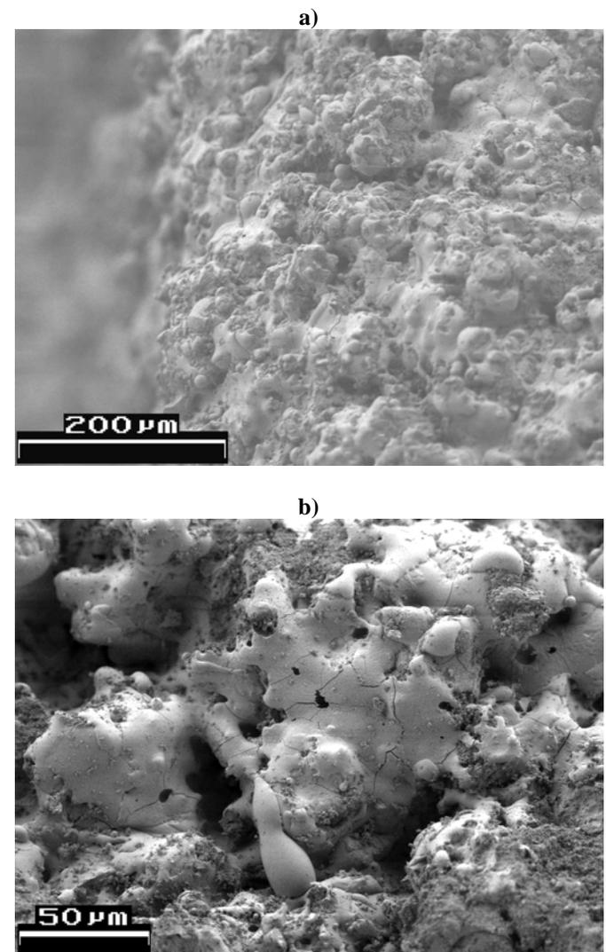
Figure 3a and 3b: SEM view of HA coating on PEEK prototype (with a tilt of 30°).
