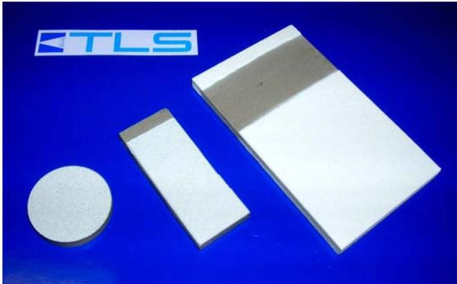
Figure 1: Coated pure PEEK disk (100  $\mu\text{m}$ ), and plates (middle: 150  $\mu\text{m}$ ; right 500  $\mu\text{m}$ ). The grey bands are uncoated surfaces (protected with specific masks during plasma spraying).
